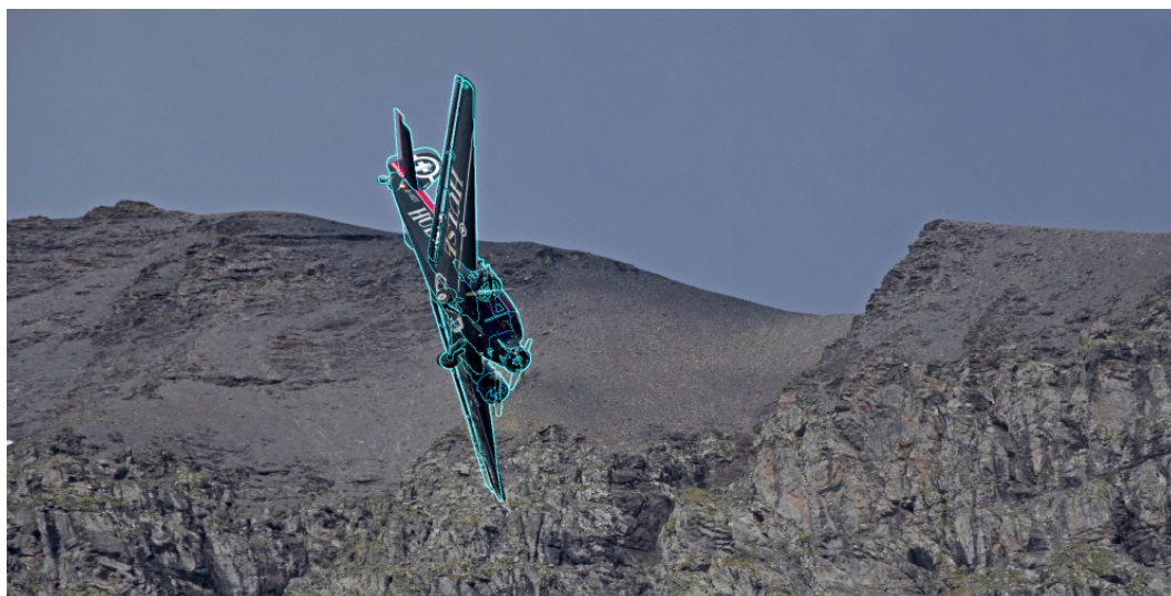
Figure 7: Image showing HB-HOT at point F16, including a superimposed three-dimensional model of an identical Ju 53/3m g4e (light blue) for the purpose of determining attitudes, wing deflection and deflections of the control surfaces. The direction of view is north-eastwards, the southern spur of Piz Segnas is visible in the background.
